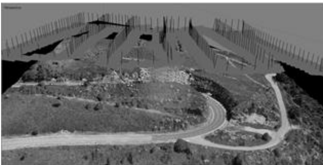
Figure 1: UAV pathing and image alignment with computed camera positions and the resulting point cloud.
